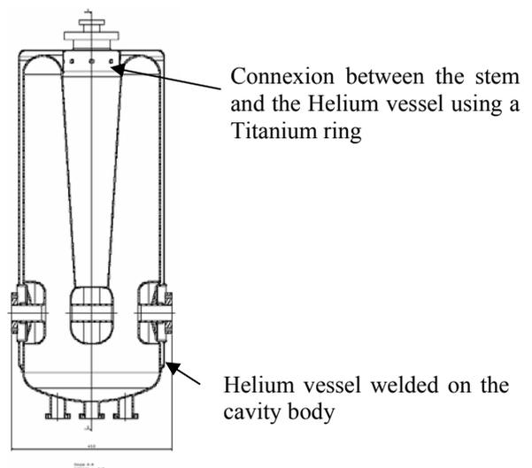
Figure 9: New design of the Helium vessel.
