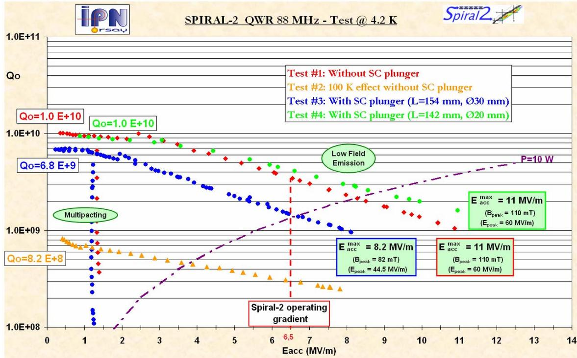
Figure 4: Cold tests results:  $Q_o$  vs.  $E_{acc}$
