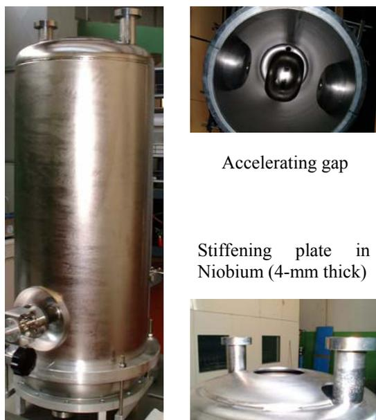
Figure 1: Beta 0.12 QWR during the fabrication
