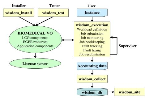
Fig. 1. Design of the WISDOM production system
