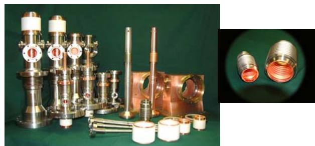
Fig. 4: Photographs of the different copper-plated parts of TTF3 coupler
