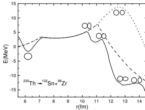
FIG. 2: Potential barrier for a  $^{230}\text{Th}$  nucleus emitting a doubly magic nucleus  $^{132}\text{Sn}$ . The dotted and dashed curves give the macroscopic energy for two-body shapes respectively within two spheres and ellipsoidal deformations. The solid line includes the shell and pairing corrections.  $r$  is the distance between mass centres.
