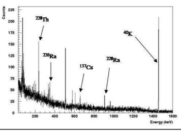
FIGURE 2. Gamma spectrum of a salt from the island of Ré.
