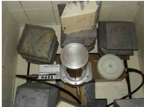
**Fig. 11: The detector with its Pb shielding**
