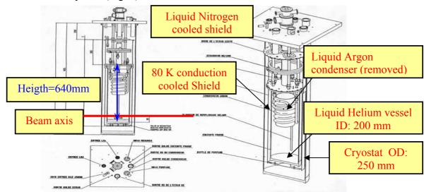
Fig.1: Drawing of the cryostat and the insert
