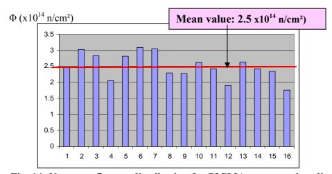
Fig. 14: Neutrons fluence distribution for PICMA actuators irradiation
