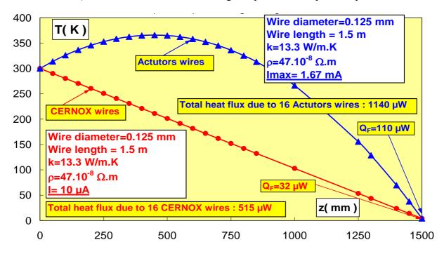
Fig. 7: Temperature profile along the manganin wires (Actuators and CERNOX).
