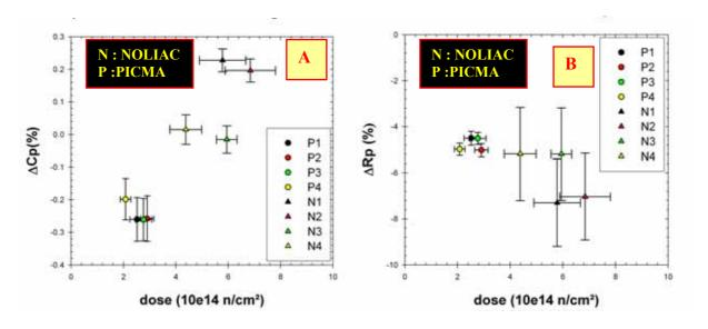
Figure 20: Effect of fast neutrons dose on capacitance (A) and parallel resistance (B) at T=4.2 K.
