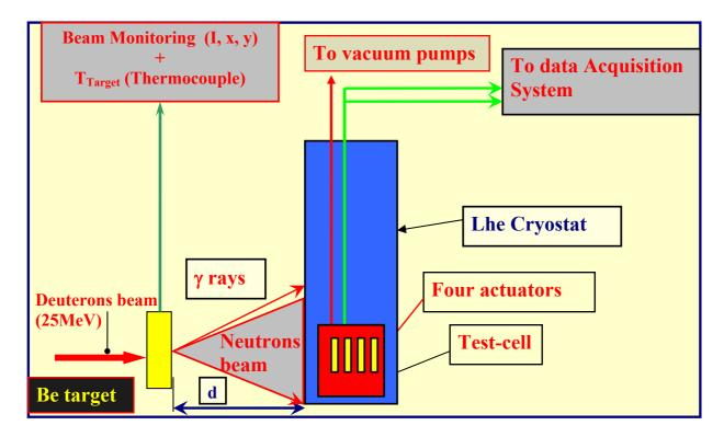
Fig. 3: Sketch of fast neutrons production process.
