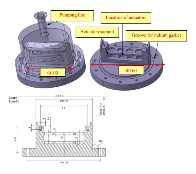
Fig. 4. Drawings of the test chamber
