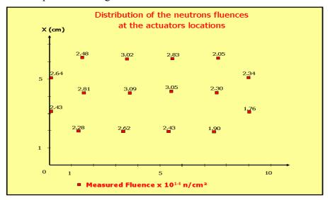
Fig. 13: Neutrons fluence map for PICMA actuators irradiation
