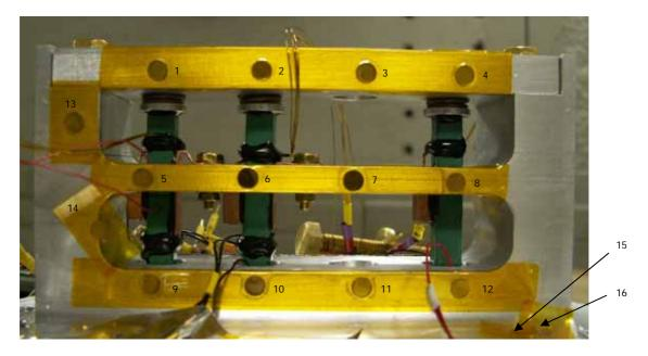
Fig. 18: Distribution of the nickel foils on the JENA piezoelectric actuators support
