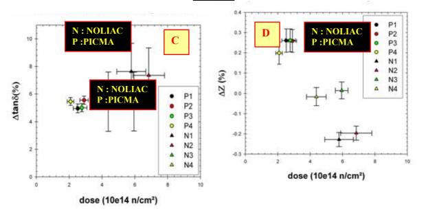
Figure 21: Effect of fast neutrons dose on loss factor (C) and impedance (B).
