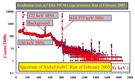
Fig. 12: Typical spectrum of nickel foil #1 (Run of February 2005)
