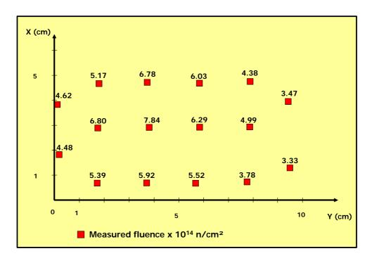
Fig. 16: Neutron fluences distribution for NOLIAC actuators irradiation
