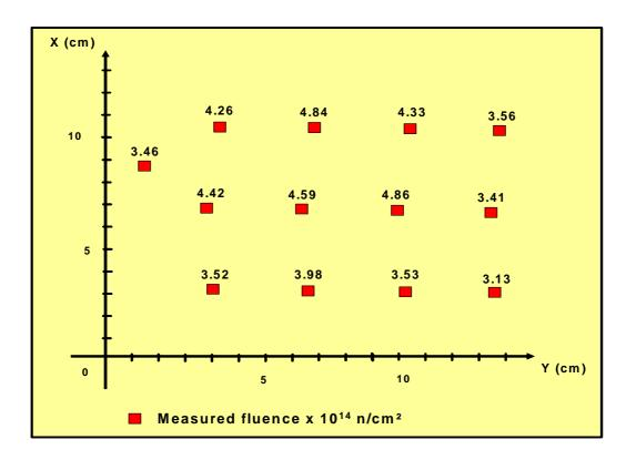
Fig. 19: Neutron fluences distribution for JENA actuators irradiation
