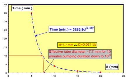
Fig. 6: Pumping duration of the test-cell in the Knudsen regime for reducing the pressure from 10<sup>-2</sup> to 10<sup>-6</sup> Torr (Material desorption not taken into account).
