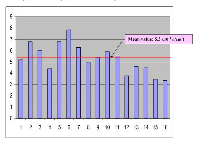
Fig. 17: Neutrons fluence distribution for NOLIAC actuators irradiation
