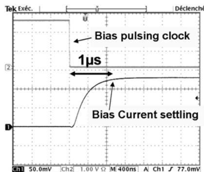
Figure 14: Analog bias fast switching results.
