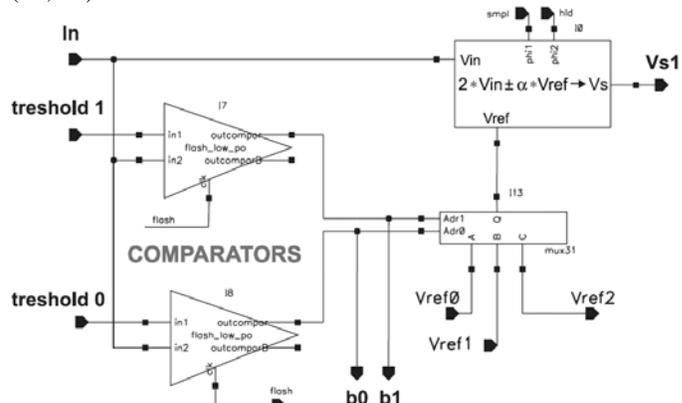
Figure 7: Bloc diagram of a 1.5bit sub-converter stage.
