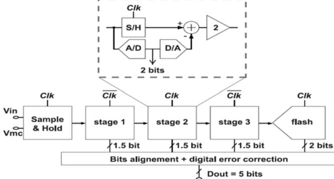
Figure 2: General block diagram of a pipelined converter.
