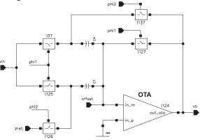
Figure 10: The capacitive precise multiplier scheme.
