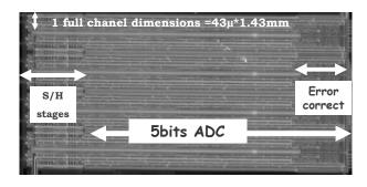
Figure 11: Layout of a prototype with 8 channel ADC.
