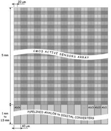
Figure 1: Sketch view of a MAPS array with a data conversion stage.
