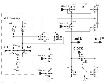
Figure 9: The comparator scheme.
