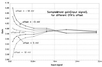
Figure 4: SHA gain according to the input signal, with the OTA's offset as a second parameter.
