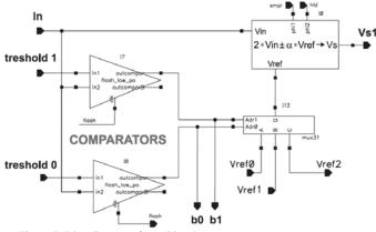
Figure 7: Bloc diagram of a 1.5bit sub-converter stage.
