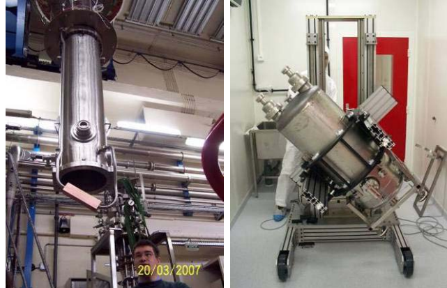
Figure 1: Cavity A and one of the 2 cavities B in the clean room with the handling robot
