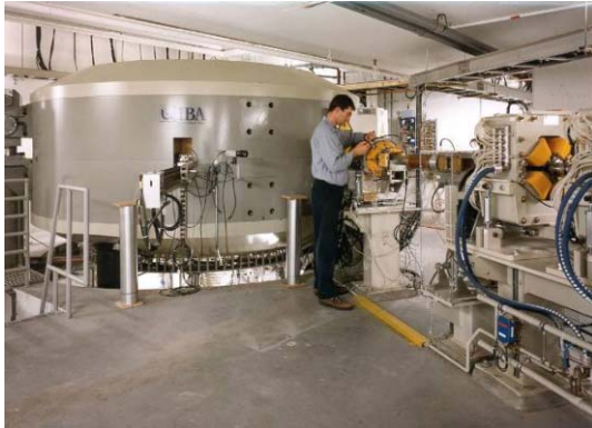
Fig. 9: IBA proteus 235 compact normal-conducting cyclotron.
