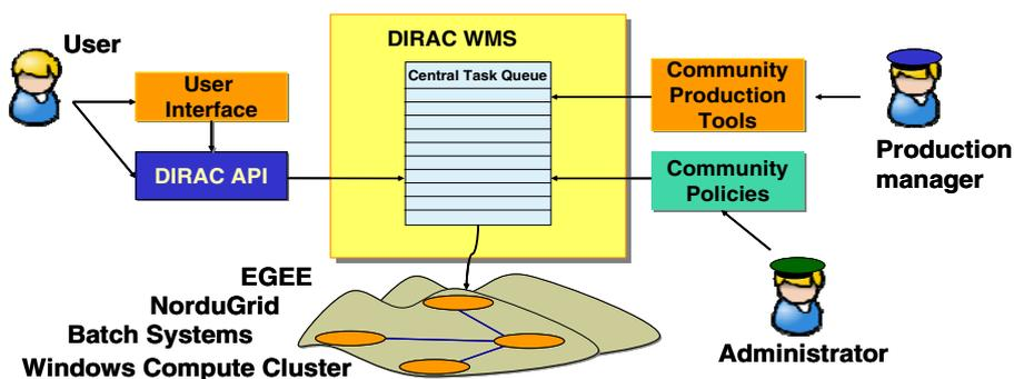
Figure 3 DIRAC WMS with the central Task Queue
