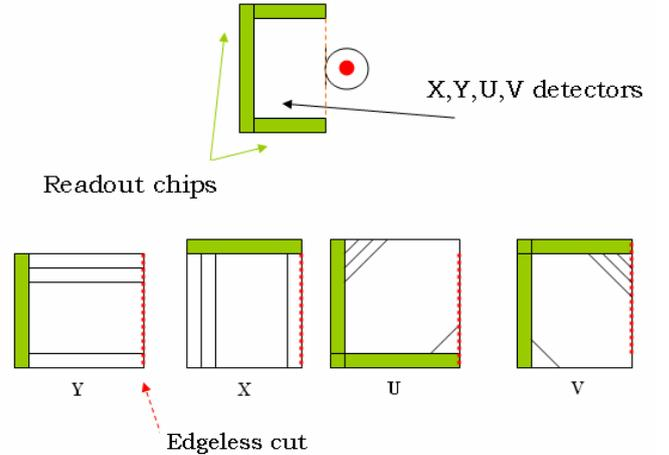
Figure 5: Detector geometries
