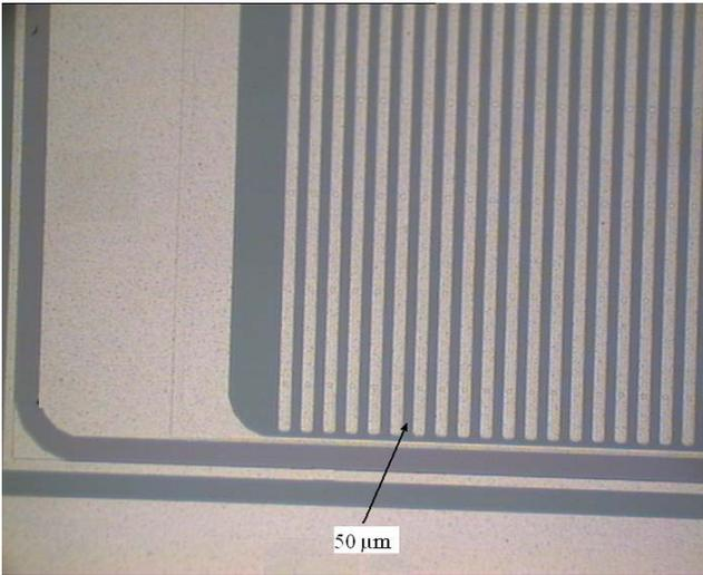
Figure 6: 50  $\mu\text{m}$  pitch detectors from CANBERRA
