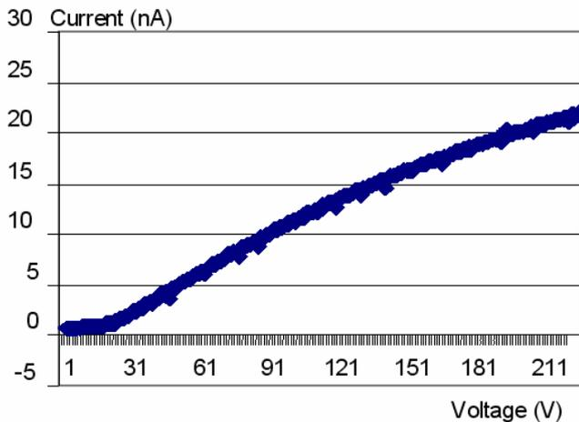
Figure 7: Reverse current (0.7 cm<sup>2</sup> detector)
