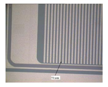
Figure 6: 50 µm pitch detectors from CANBERRA
