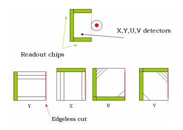
Figure 5: Detector geometries
