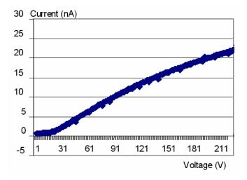
Figure 7: Reverse current (0.7 cm2 detector)
