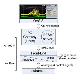
Figure 1 System architecture
