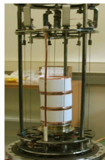
Fig 3. TiN evaporation bench. A column of three alumina windows is installed.
