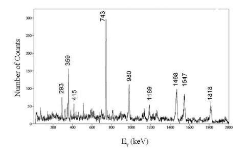
Figure 10. The  $\gamma\text{-ray}$  spectrum of the 2pn  $^{45}\text{Ti}$  fusion channel with a gate on the 586 keV  $\gamma$  peak.
