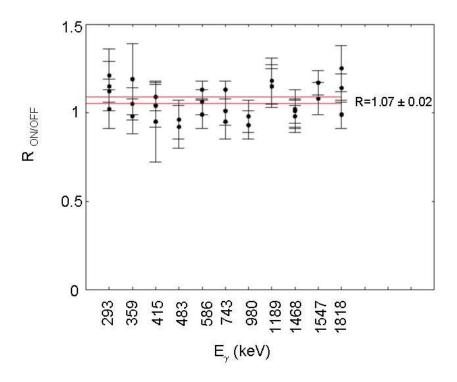
Figure 11. The ON/OFF resonance ratio of the  $\gamma$ -ray intensities for the indicated transitions in <sup>45</sup>Ti. For a given  $\gamma$ -ray energy, the values of R have been obtained using different gating cascade transitions.
