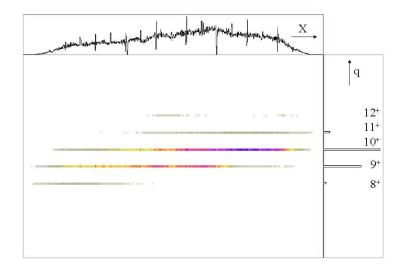
Figure 2. The  ${}^{24}Mg$  fragments: position X on the focal plane versus charge state distribution q.
