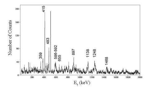
Figure 8. The  $\gamma$ -ray spectrum of the 2pn  $^{45}$ Ti fusion channel with a gate on the 293 keV  $\gamma$  peak.
