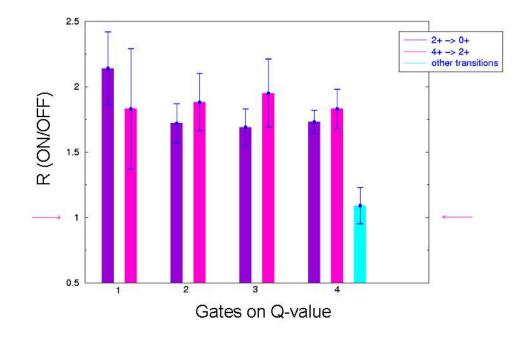
Figure 5. ON and OFF yield ratios R for different <sup>24</sup>Mg transitions and Q-value gates.
