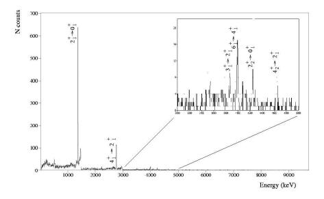
Figure 3. Gamma spectrum of the  ${}^{24}Mg + {}^{24}Mg$  reaction recorded in coincidence with  ${}^{24}Mg$  fragments.
