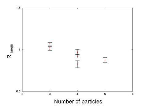
Figure 14. Average of the ON/OFF resonance ratio for the fusion-evaporation channels as a function of the number of emitted particles.
