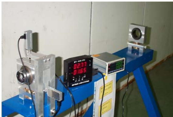
Figure 13: Laser alignment under test
