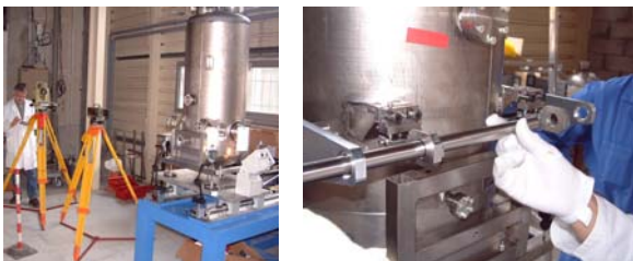
Figure 12: Axis located on the helium tank with respect to the measured cavity axis
