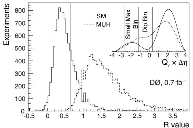
FIG. 4: Distributions of the  $R$ -test statistic for the SM ensembles (solid line) and the MUH ensembles (dashed line). The vertical line indicates the measured value from the data. The inset plot indicates the positions of the two bins used for the  $R$ -test as determined by a fit to the SM  $Q_\ell \times \Delta\eta$  distribution (solid line). For comparison, a fit to the MUH  $Q_\ell \times \Delta\eta$  distribution is shown as the dashed line.
