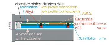
Figure 6: AHCAL integrated layer
