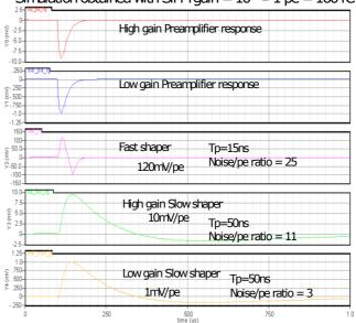
Figure 9: One channel simulation
