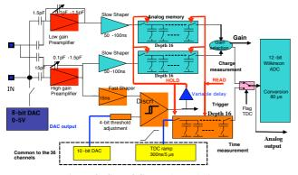
Figure 8: SPIROC one channel diagram
