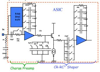
Figure 2: FLC\_SiPM : one channel architecture
