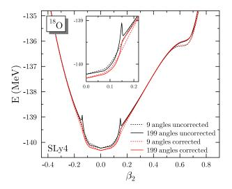
FIG. 10: (Color online) Particle number restored energy  $\mathcal{E}^N$  as a function of quadrupole deformation without and with regularization of all bilinear terms in the EDF, including the quadratic part of  $\mathcal{E}^{\rho\rho\rho^{1/6}}$ . Results are shown for two different numbers of discretization points in the computation of the integrals over the gauge angles.
