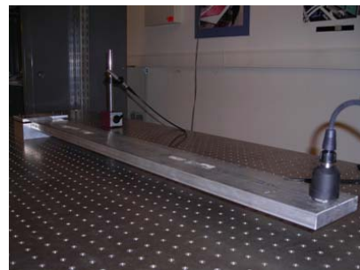
Figure 5: Canteliver beam instrumentated with two accelerometers and two microphones
