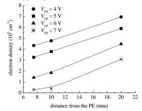
**FIGURE 2.** Variation of electron density with distance from the plasma electrode, for four values of the plasma electrode bias  $V_{PE}$ .
