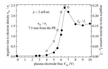
**FIGURE 9.** Ratios of the negative ion to electron density (dashed line) and the extracted negative ion to electron current (solid line) *vs.* plasma electrode bias. <sup>4</sup>
