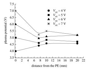
FIGURE 5. Variation of the plasma potential with distance from the plasma electrode, for four values of the plasma electrode bias  $V_{PE}$ .
