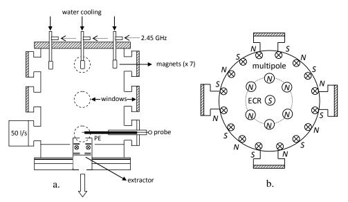
FIGURE 1. Schematic representation of the ECR-driven hybrid multucusp source Camembert III (a) and the magnets forming the multicusp configuration (b).
