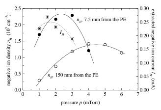
**FIGURE 7.** Comparison between the negative ion density close to the extractor aperture (solid symbols) and at the center of the source (open symbols) *vs.* pressure. The extracted negative ion current is also compared (dotted line).<sup>4</sup>
