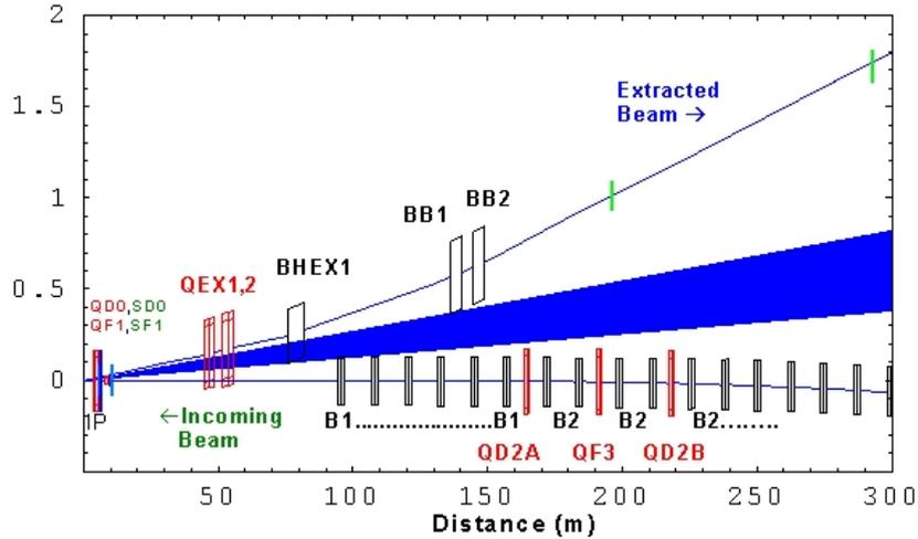
Figure 1: Schematic layout of the 2 mrad ILC extraction line.
