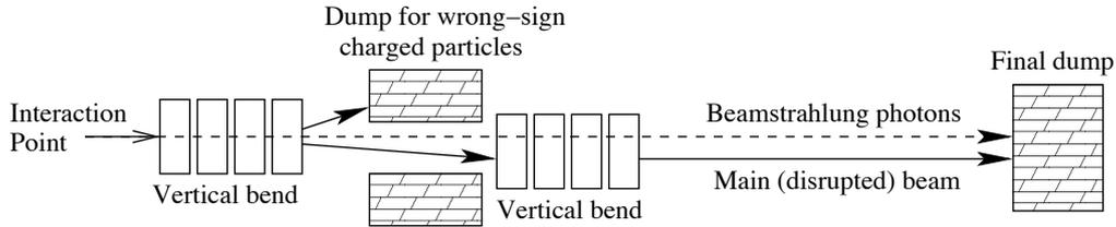
Figure 3: Schematic layout of the CLIC post-collision line.
