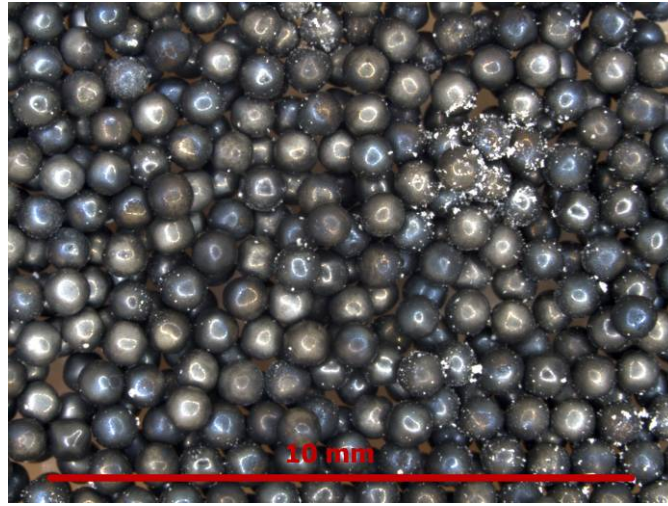
Figure 3: Photograph of SiC surface TRISO after compact oxidation at 1100 K during 16 h
