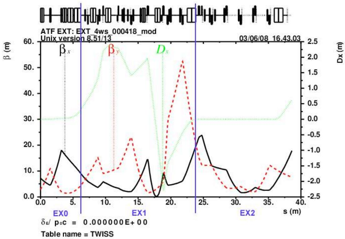
Figure 3: Optics calculation of the ATF EXT line.
