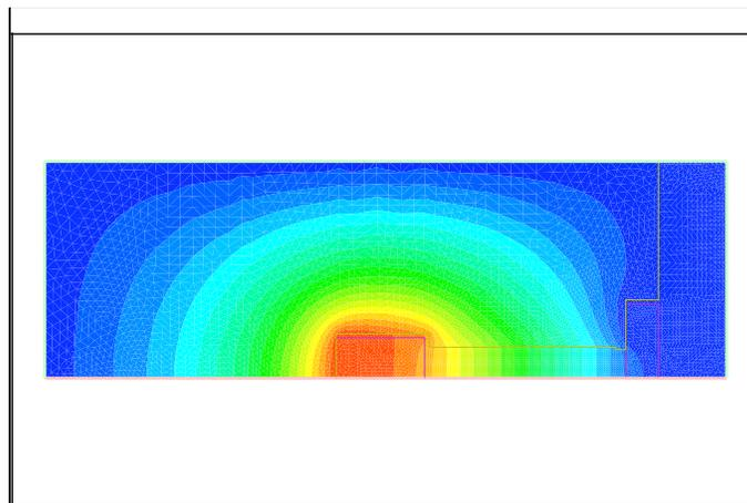
Figure 13: BS1X B field lines computed with PRIAM
