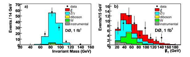
FIG. 1: Comparison of the expected distributions from backgrounds and  $t\bar{t}$  ( $m_t = 170$  GeV) in the  $\ell$ +track channels. (a)  $M_{\ell t}$  for the e+track channel without the requirement of the b-tag and with inverted  $\not{E}_T$  cuts. (b)  $\not{E}_T$  for the sum of both  $\ell$ +track channels, again without the b-tag requirement. We assume  $\sigma_{t\bar{t}} = 7.0$  pb.
