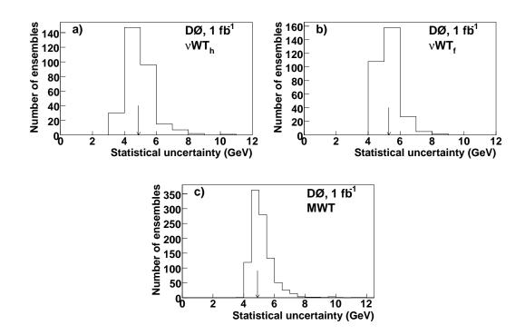
FIG. 10: Distribution of statistical uncertainties for top quark mass measurements of pseudoexperiments for the combination of all channels for simulated events with  $m_t = 170$  GeV for the (a)  $\nu WT_h$ , (b)  $\nu WT_f$ , and (c) MWT methods. The uncertainties are corrected by the calibration curve and for the pull width. The arrows indicate the statistical uncertainties for the measured top quark mass.
