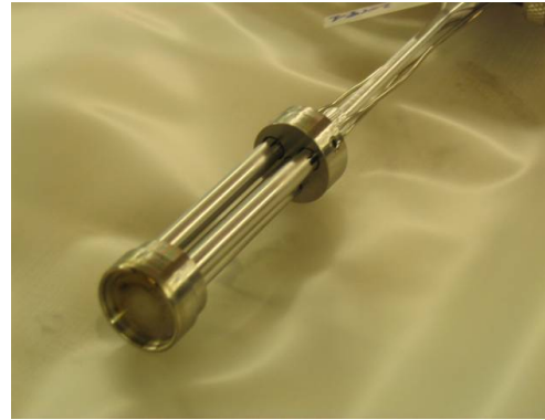
Fig. 10: Photography of a triple deposit fission chamber (CFUT-C7).
