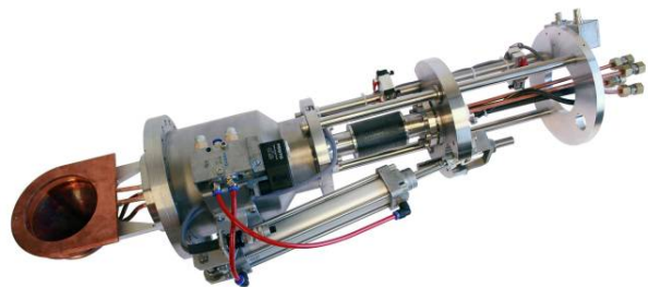
Figure 2: Photograph of the Faraday Cup of the L.E.B.T.
