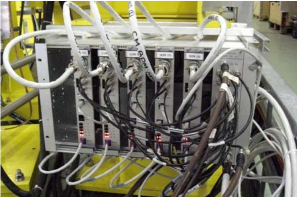
Uranus crate in CLEX with 5 chained DFE boards and one distribution board.
