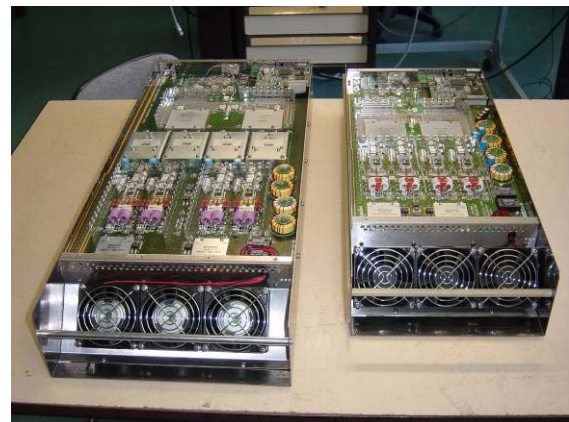
Figure 6: air-cooled 1 kW rack with and without circulators (@ ECRESO)
