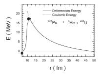
FIG. 1: Potential barrier of  $\alpha$  emission from <sup>238</sup>Pu with (solid line) and without (dotted line) the proximity energy.
