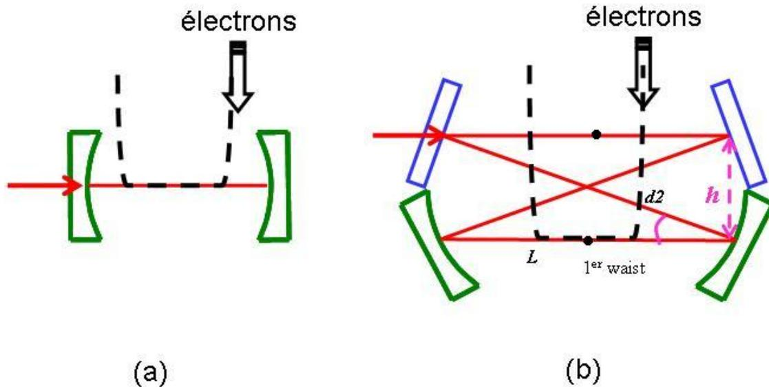
Figure 6 : (a) two-mirror cavity, the mirrors are spherical. (b) 2D bow-tie four-mirror cavity, the two upper mirrors are flat and the two lower ones are spherical.
