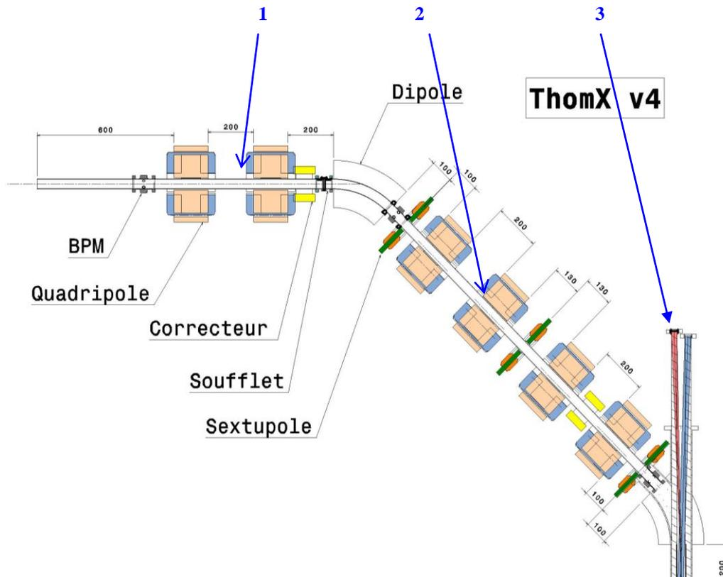
Figure 40 : Implantation of the ion pumps on a quarter of the ring with the optical cavity.
