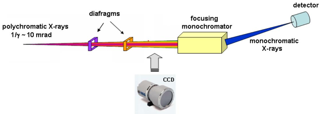
Figure 43 : Principle of the X-ray beam characterisation.
