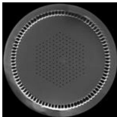
Figure 3 : rod-type photonic crystal fibre.
