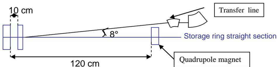
As the needed deviation is important, it has to be realized using two pulsed magnets: a thin septum magnet, insuring the most part of the deviation, and a very fast kicker which puts the injected beam on axis.
