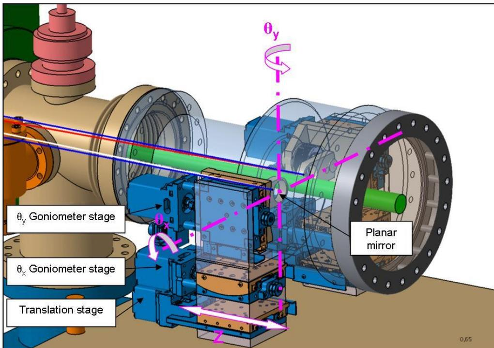
Figure 13 : Schematic view of the mirror actuators.
