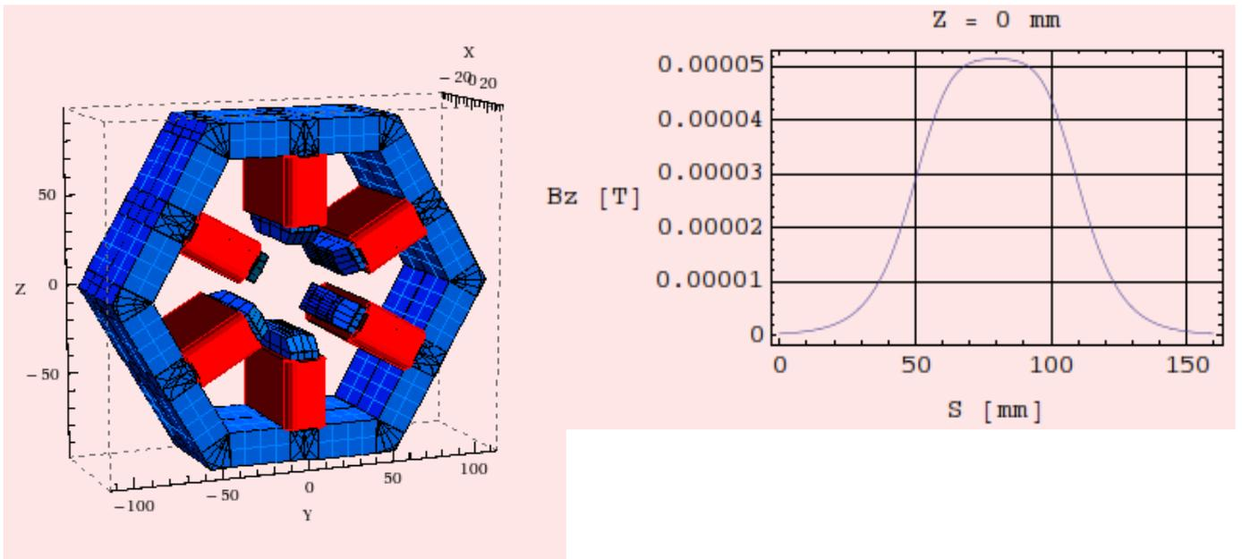
Figure 30 : Sextupole yoke and longitudinal field profile
