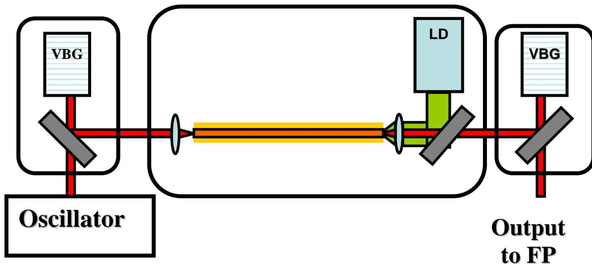
Figure 4 : Architecture of the fibre chirped pulse amplifier
