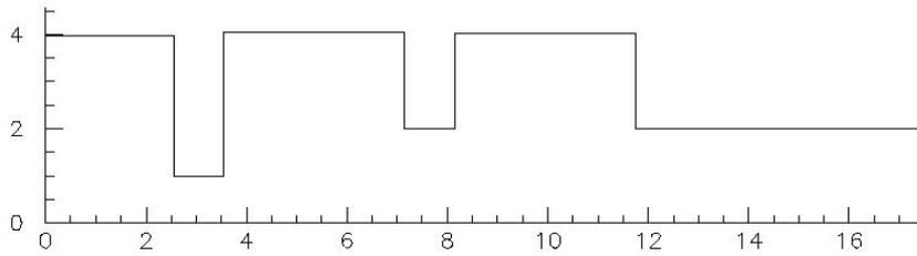
Figure 1: SUPERFISH 2D (cylindrical symmetry) model of the RF gun, vertical axis stands for the radius in cm and horizontal axis is the longitudinal symmetrical axis in cm.
