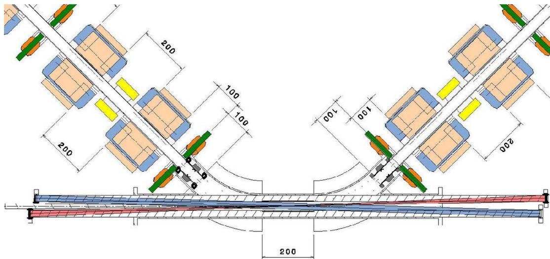
Figure 12 : Schematic location of the 2D laser cavity.
