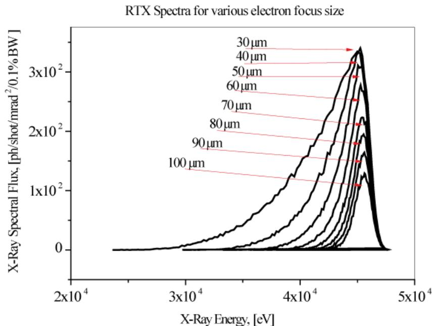
Figure 12 : On-axis spectra calculated for various electron waists sizes and head-on collision. Electron energy is equal to 50 MeV.
