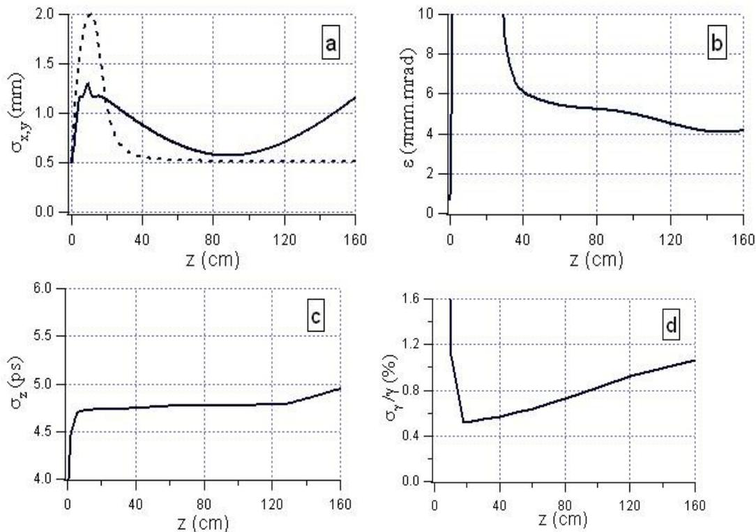
Figure 2 : PARMELA simulations, the length of the RF gun is 20 cm, the downstream distance is a drift space. All plots are r.m.s. values as a function of the distance  $z$  along the accelerator. a), beam sizes (it is the same curve either in x or in y), the dashed line stands for a schematic of the magnetic field; b), normalized emittance; c), bunch length; d), energy spread.
