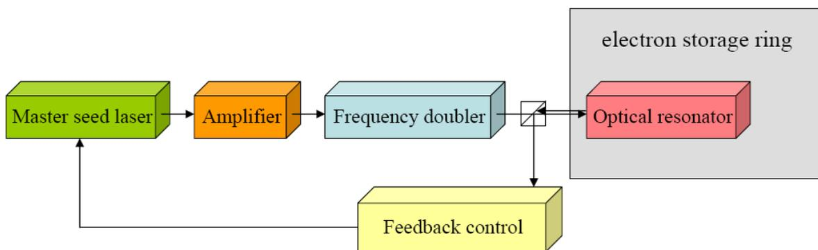
Figure 1: Block diagram of the general optical setup.
