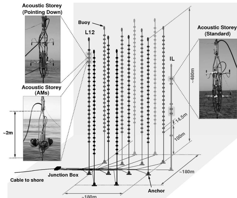
Figure 1. A sketch of the ANTARES detector. The six Acoustic Storeys are highlighted and their three different setups are shown. L12 and IL denote Line 12 and the Instrumentation Line, respectively.
