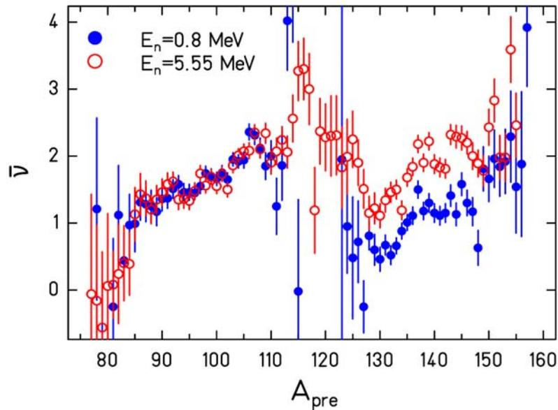
**Figure 1 :** (Colour online) Average number of prompt neutrons as a function of the primary fragment mass for the neutron-induced fission of  $^{237}\text{Np}$  at two incident neutron energies, data taken from ref. [14].
