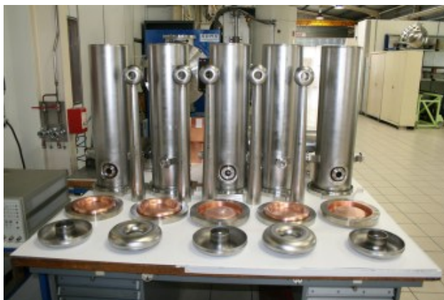
Figure 2: Series cavities just before tuning operation in the manufacturer premises.
