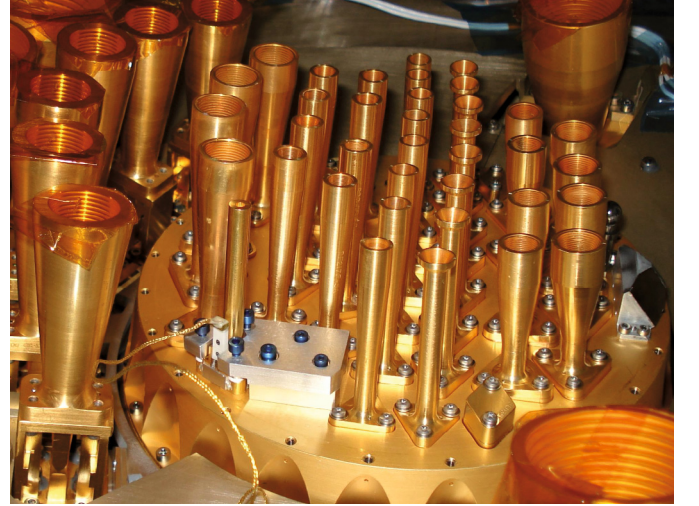
Fig. 5. One can see the HFI and the LFI horns on this picture taken during ground tests of the Proto-Flight Model. An additional horn, mounted for alignment tests, is visible at the end of the 100 GHz row.
