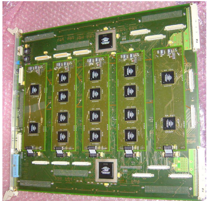
Fig. 11. BFU motherboard, equipped with daughterboards. The white 50-pin connectors are the neighbor connections to the second board. The blue connector on the left connects to the VME controller board. The small FPGAs implement the BFU algorithm, the two large ones the PSU algorithm.
