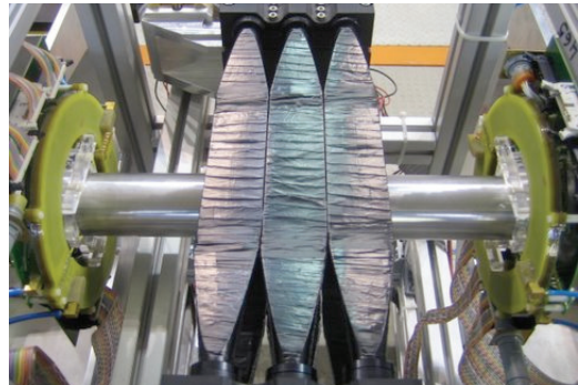
Figure 3: Gem ring (left, right) and SIDDHARTA scintillator K-Monitor (center) mounted on DAFNE IR.
