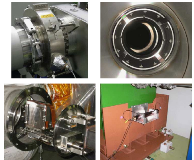
Fig. 4. Photographs of the primary beamline monitors. Upper left: CT. Upper right: ESM. Lower left: SSEM. Lower right: BLM.
