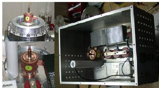
Figure 6: The HV module connected with feed-through.
