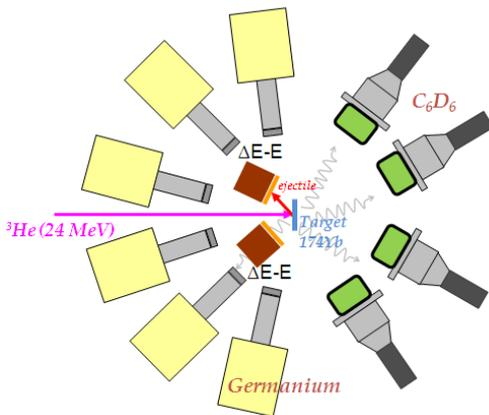
Fig. 2 : Top view of the experimental set-up for radiative capture probability measurements. The four  $\text{C}_6\text{D}_6$  liquid scintillators were placed at forward angles with respect to the beam direction, whereas the two Si telescopes and the
