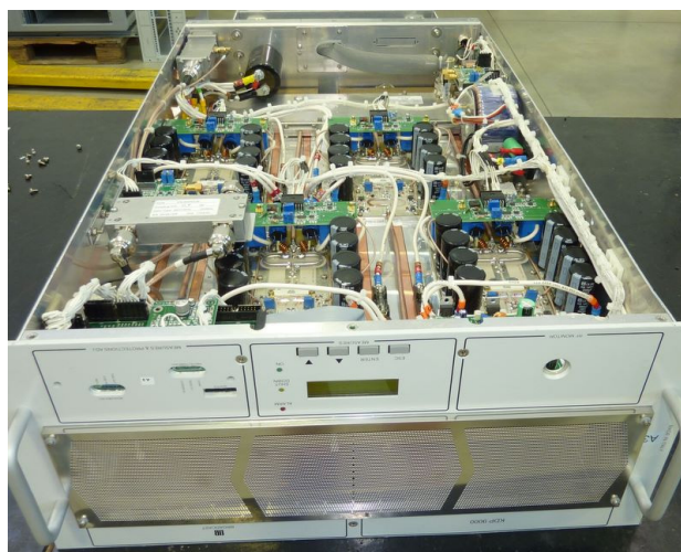
Figure 2: 7 kW amplifier unit.
