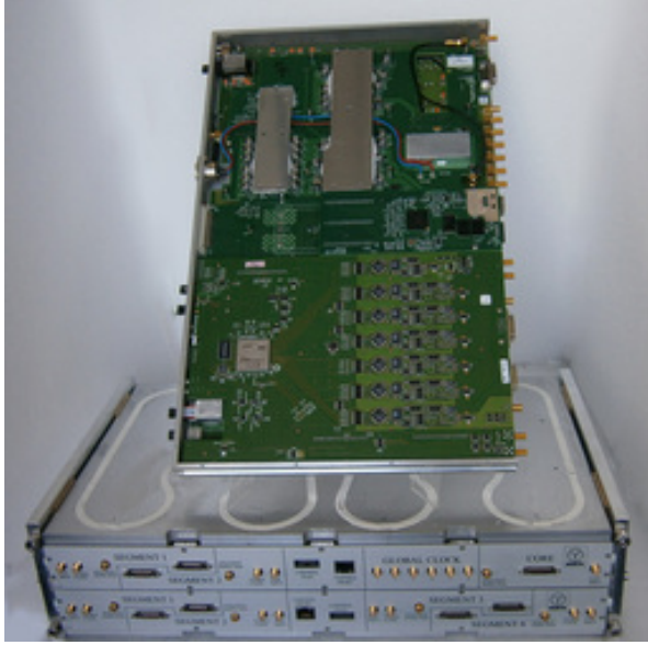
Figure 25: (Colour online) Photograph of the AGATA digitiser.
