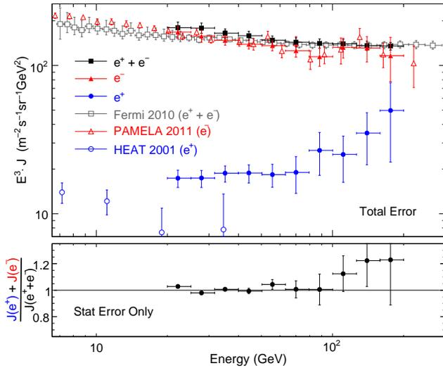
FIG. 4: Energy spectra for  $e^+$ ,  $e^-$ , and  $e^+ + e^-$  (control region). In the control region where both species are allowed, this analysis reproduces the Fermi LAT results reported previously for the total electron plus positron spectrum [20, 21] (gray). Previous results from HEAT [9] and PAMELA [38] are shown for reference. The bottom panel shows that the ratio between the sum and the control flux is consistent with 1 as expected.
