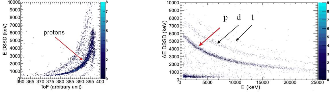
Figure 2: Proton identification in MUST2 telescopes. Left: Energy versus Time of Flight (ToF) selection, where ToF is measured with respect to CATS detector; data of 2 telescopes are summed. Right:  $\Delta E$ -E selection, where  $\Delta E$  is the energy loss of particles in the first layer of MUST2 detectors, and E the energy deposit of particles in the Si(Li) detector; data of 3 telescopes are summed.
