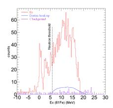
Figure 3: Left: Experimental kinematic lines energy versus angle for  $d(^{60}Fe,p\gamma)^{61}Fe$  reaction in the laboratory frame; calculated kinematic lines for the 207 keV (in red) and 2160 keV (in black) excited states are plotted for comparison. Right: Excitation energy spectrum of  $^{61}Fe$ ; Carbon background and break-up component are shown.
