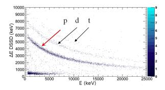
Figure 2: Proton identification in MUST2 telescopes. Left: Energy versus Time of Flight (ToF) selection, where ToF is measured with respect to CATS detector; data of 2 telescopes are summed. Right:  $\Delta E$ -E selection, where  $\Delta E$  is the energy loss of particles in the first layer of MUST2 detectors, and E the energy deposit of particles in the Si(Li) detector; data of 3 telescopes are summed.
