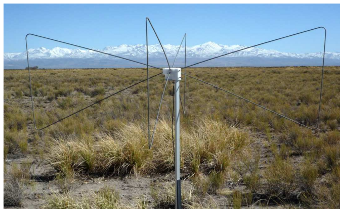
Figure 1: The Butterfly antenna, a dual polarization active antenna using an isosceles triangle as antenna radiator element, and a dual channel LNA located in a plastic mechanical frame placed at the antenna feedpoint.
