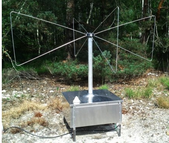
Figure 4: A Butterfly antenna installed at the site of the Nançay Radio Observatory. The antenna construction aims at a close integration with a box containing the readout electronics and a center pole which is also used to carry an antenna for wireless communication.
